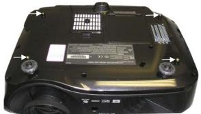
1. Locate the mounting points on the bottom of the projector (see arrows above for mounting point recognition).
